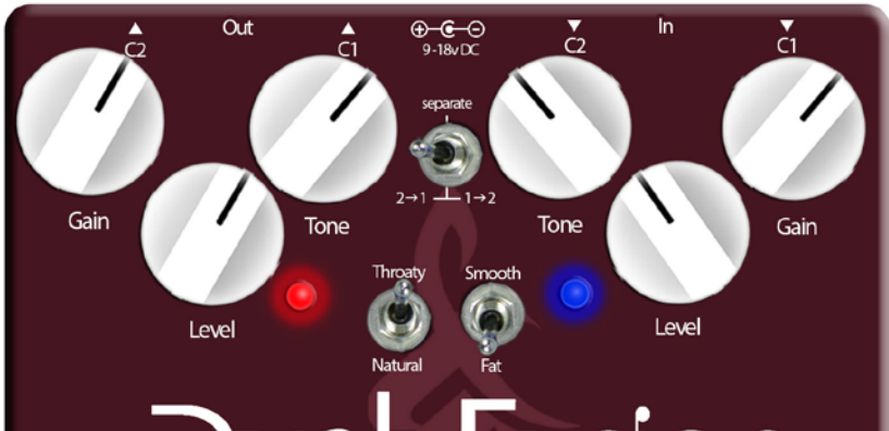
Channel 2 into 1 Input: Channel 2 Output: Channel 1 Switch: 2 → 1
